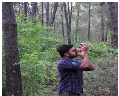
Image 17: Estimation of tree height with help of Abney's level
